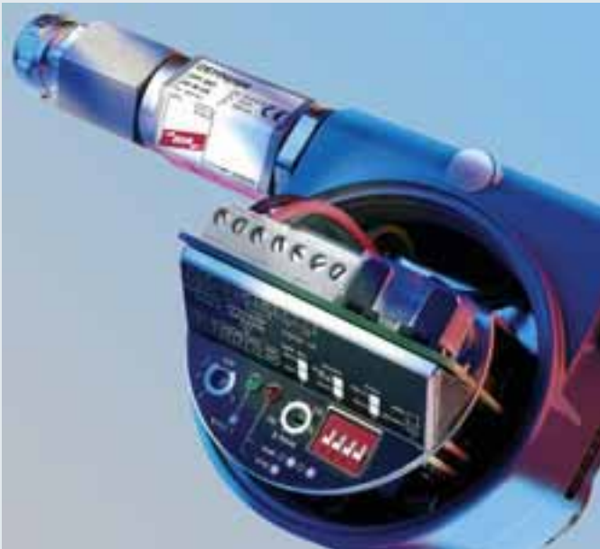
Surge arrester for outdoor use for screwing into 2-conductor process field devices. Stainless steel, IP 67.
