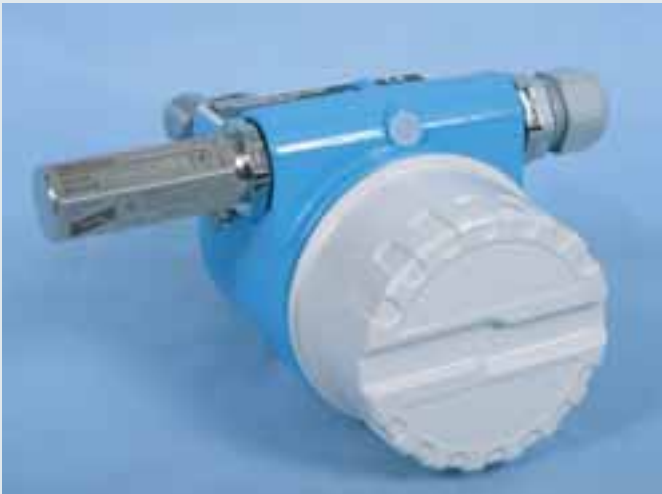
Surge arrester for outdoor use for screwing into 2-wire process field devices. Stainless steel, allows for installation up to IP 67.
