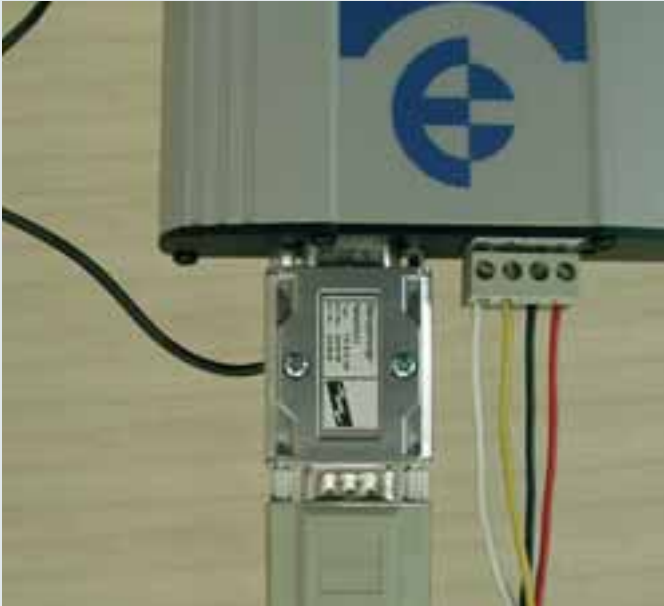
Surge protective adapter, D-SUB plug-in connection, socket-pin type.
